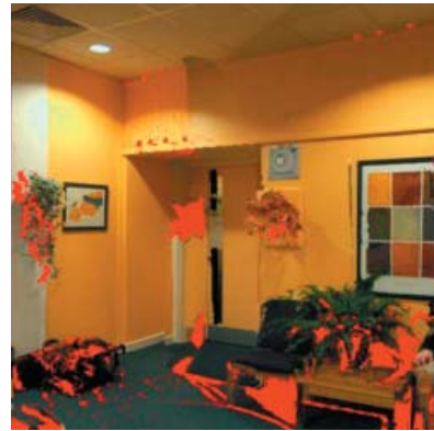
The model set shown left is rendered with view-dependent texture mapping. Areas occluded from the laser are shown in red.
